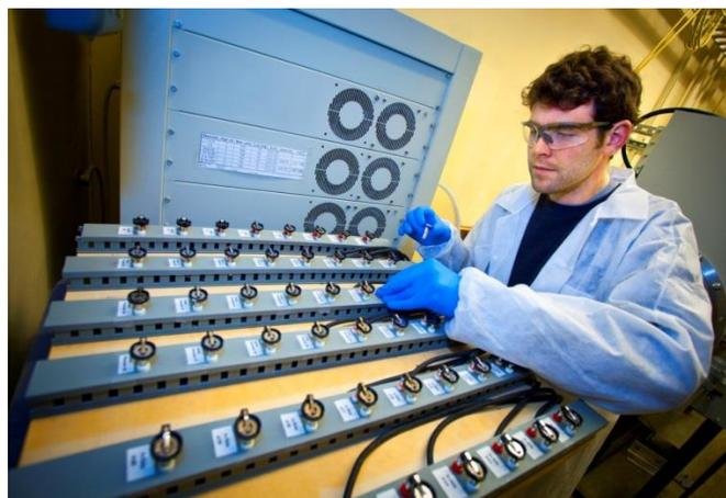
Figure 7. Loading a lithium coin cell for testing on an Arbin battery cycler at the Lawrence Berkeley National Laboratory [25]
